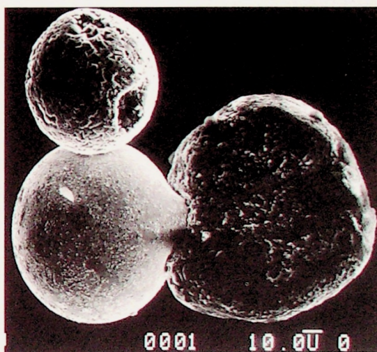
7 Fig. 7 - SEM picture of an undeformed pyrrhotite crystal showing a marked polygonal structure on the surface due to an oxidation which is stronger than that shown by the pyrite given in Fig. 6.
